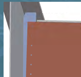
Cambered position Back view showing girders rotated up from horizontal plane Diaphragms not aligned (designed to fit in final position)
